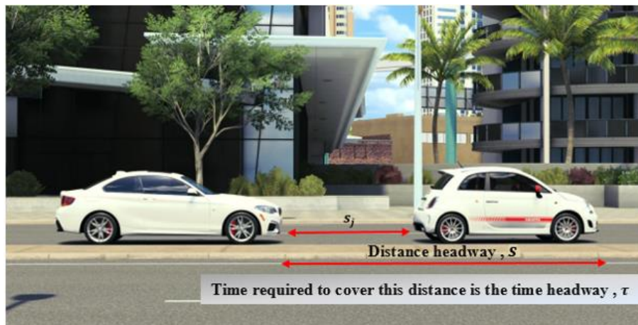
Figure 2.1 The distance and time headways between leading and following vehicles.
