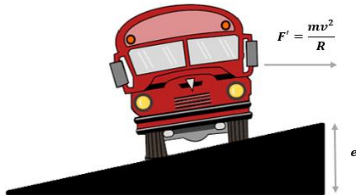
Figure 5.2 Centrifugal force and highway superelevation.
