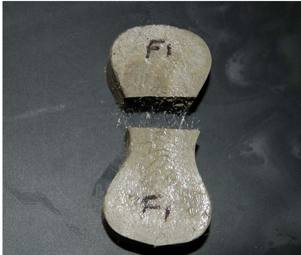
Figure 8 - A Tested Specimen Showing Polypropylene Fibers Across the Crack
