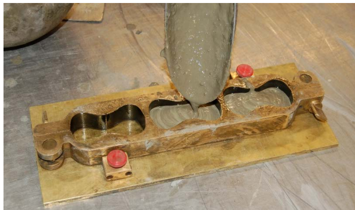
Figure 2 - Molds for Casting Briquette Specimens
