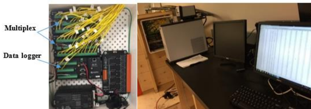
a) Data acquisition system b) Data acquisition system connected with a personal computer
