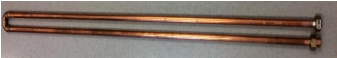
a) Conventional U-Tube pipe configuration.
