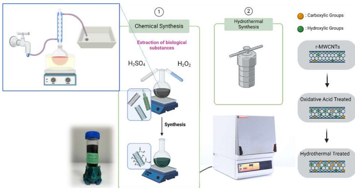
Figure 3-1 The protocol for Synthesizing surface-oxidized MWCNTs
