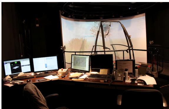
Figure 10: CAREN Technician's Station Behind the Machine
