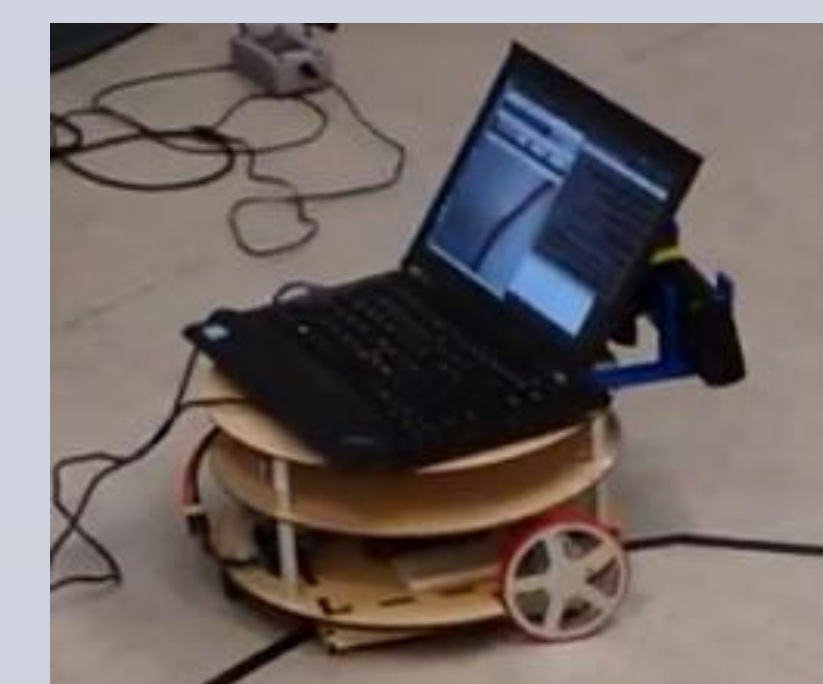
Fig 11. AMR Performing Line Following
