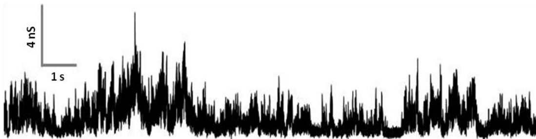
Figure 3-26: Representative trace of erratic (purple) type activity for the compound \bar{\text{OOC-Hex-ADip-Oct-SH}} ( 3-71 ). Conditions: diPhyPC bilayer, 250 \mu\text{M} diameter aperture, Ag/AgCl electrodes, KCl junction solution and salt bridges, 1M CsCl with 10mM each of TRIS and HEPES as buffer, applied potential +150 mV.
