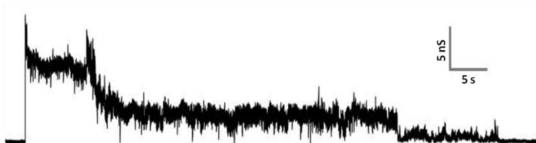
Figure 3-24: Representative trace of multi-level (blue) type activity for the compound \bar{\text{OOC-Hex-ADip-Oct-SH}} ( 3-71 ). Conditions: diPhyPC bilayer, 250 \mu\text{M} diameter aperture, Ag/AgCl electrodes, KCl junction solution and salt bridges, 1M CsCl with 10mM each of TRIS and HEPES as buffer, applied potential +150 mV.
