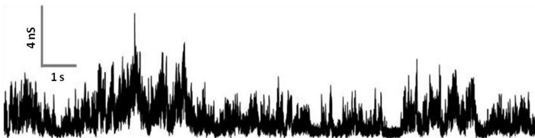
Figure 3-21: Representative trace of erratic (purple) type activity for the compound \bar{\text{OOC-Hex-ADip-Oct-S-Hex-OH}} ( 3-59 ). Conditions: diPhyPC bilayer, 250 \mu\text{M} diameter aperture, Ag/AgCl electrodes, KCl junction solution and salt bridges, 1M CsCl with 10mM each of TRIS and HEPES as buffer, applied potential +150 mV.
