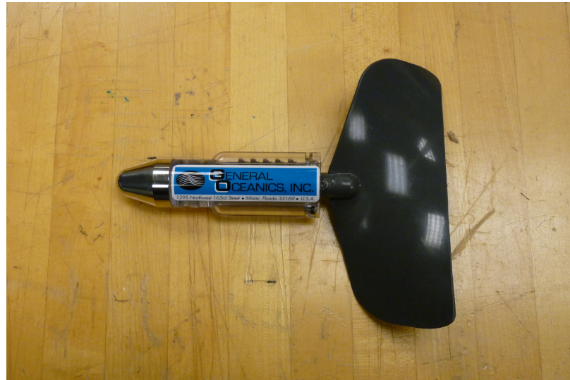
Figure 3.10 – The flowmeter used to measure ambient water velocity.
