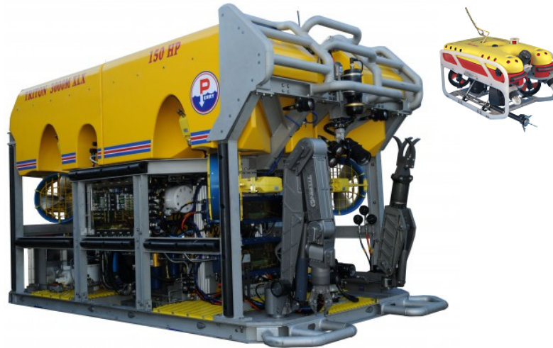
Figure 1.1 – Approximate size difference between the XLX 150HP work class ROV (left) and the Seacye Falcon observation class ROV (right).
