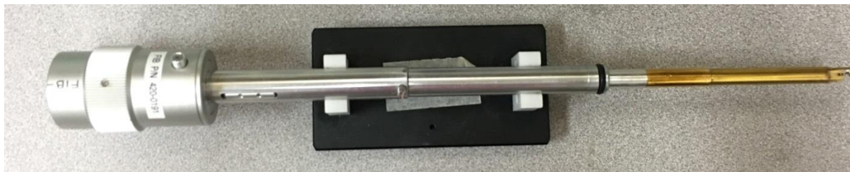
Figure A.6: TEM sample holder inserted into FIB in order to attach the specimen into the viewing area
