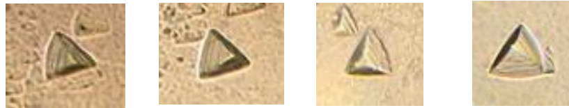
Figure 3.18: Examples of etch pits representing tetrahedral slide systems observed during the experiment in both (111) and (211) oriented CZT samples
