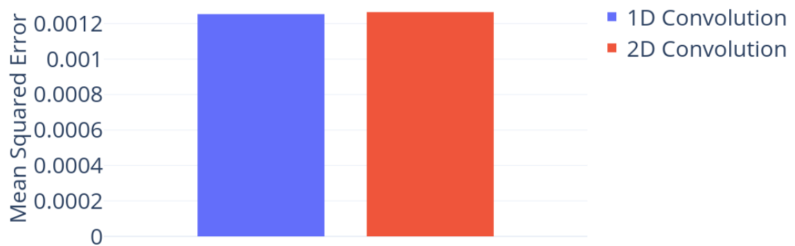
Figure 3.3: Performance comparison between one dimensional convolution and two dimensional convolution. There's no evidence showing we should use two dimensional convolution over one dimensional convolution.
