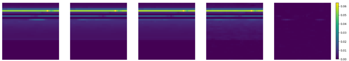
(a) ResNet based model single frame extrapolation visualization on the test data (Input1, input2, ground truth, synthesized frame, residual plot. Left to right)
