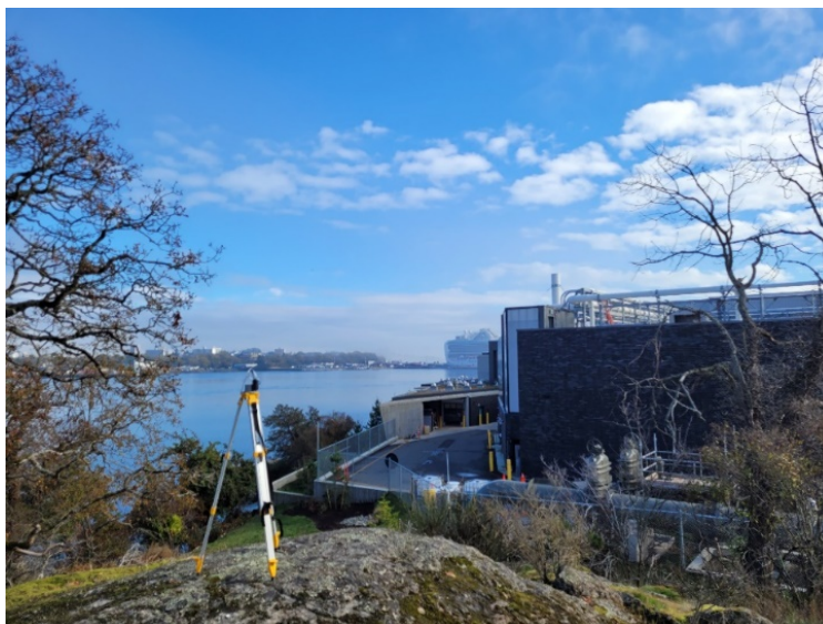
Figure 12: Photo of deployment at fence line of WWTP3 using sorbent tubes for collection of air samples, seen mounted on tripod.
